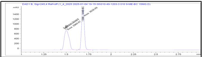
Note: Peak at 1.5 min. is matched with the method extraction solvent.
